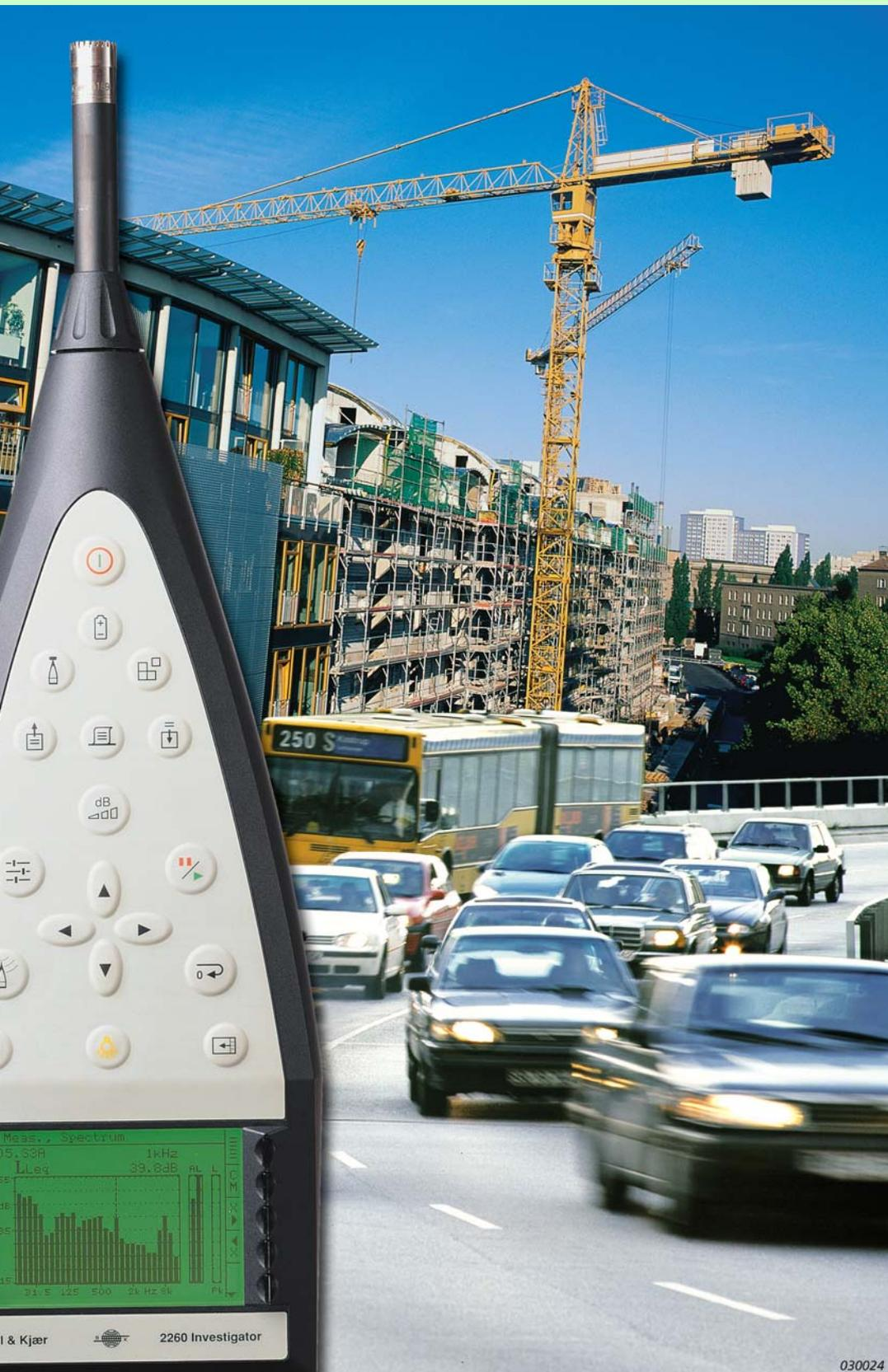
2260 Investigator™ is a battery-operated, hand-held, programmable sound analyzer. Its embedded operating system, based on a PC architecture, is closely integrated with a digital signal processor (DSP) and two-channel microphone conditioning electronics, all together creating a versatile platform for high-quality real-time sound analyses.
