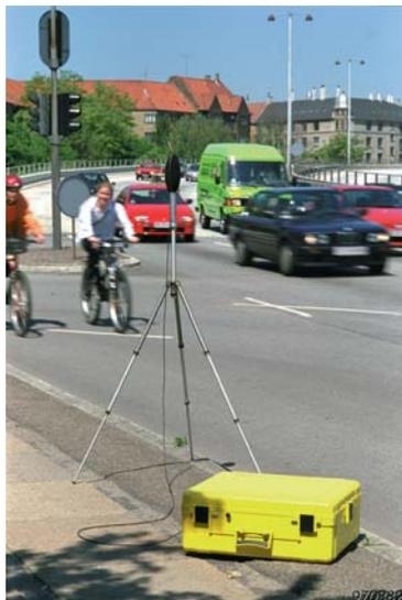
For noise monitoring in out-of-the-way places, Outdoor Gear Type 3592 offers security and weather-protection for 2260 Investigator. The modular system consists of a weatherproof case, outdoor microphone kit, microphone extension cable, microphone tripod or mast, sealed lead-acid battery, charger for battery, DAT recorder (not supplied by Brüel & Kjær), and cables for interconnection.
