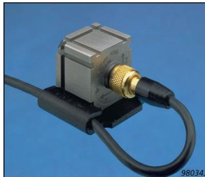
Special effort has been put into making mounting as flexible as possible. The accelerometer housing has slots that allow the use of mounting clips so that the accelerometers can be easily fitted to a number of different test objects, or removed, for example, for calibration. UA 1408, UA 1473 and UA 1474 are sets of one hundred plastic mounting clips. UA 1563 is a set of five high-temperature clips.
