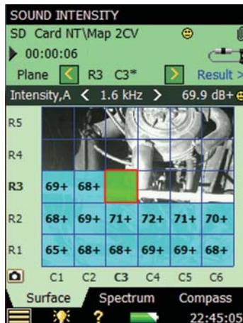
During the measurement you can use the Surface View for housekeeping. The coloured segments on top of the image of the measurement object are ideal for keeping track on the measurement process.
