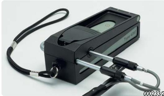
Complete calibration can be made using a Sound Intensity Calibrator Type 4297. This includes pressure calibration of both channels, phase calibration of the two channels and verification of the pressure-residual intensity index. Phase calibration enhances the dynamic capability and extends the usable frequency range down to 50 Hz using a 12 mm spacer.
