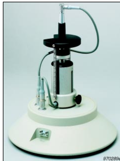
Fig. 5 Microphone fixture showing set-up with a 1/2" microphone. Notice that the collar around the main stem is much lower than that in Fig. 4
